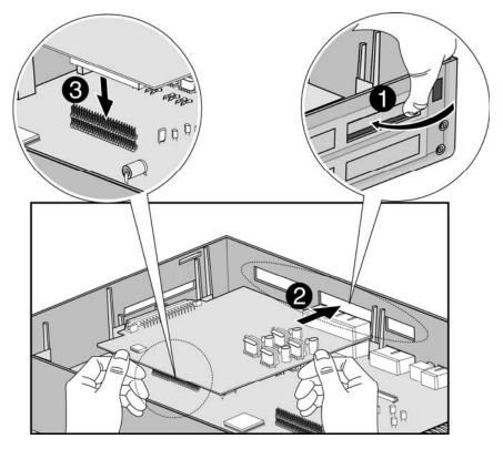
Figure 3.1 Board Installation
